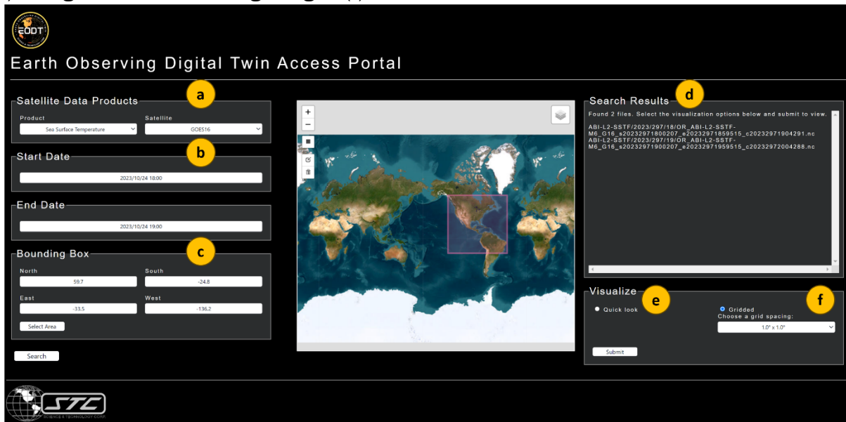
Figure 1.15 Web portal that has the user interface to search the NODD. Users can query the archive by (a) data product and satellite, (b) date and time, (c) geolocation bounding box. After clicking “search” in the lower left, the portal returns a list of filenames (d) that match the query. The user can then visualize the data in its (e) native grid using “quick look” or (f) regrid the data to a regular grid of their choice.
