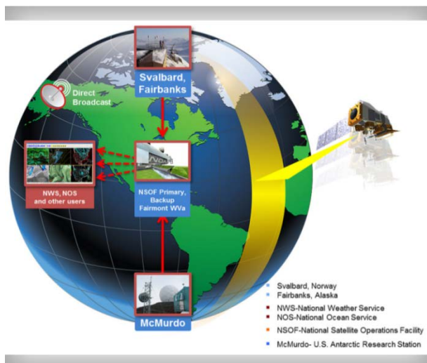
This image show the Suomi NPP versatile ground system that controls the spacecraft, ingests and processes data and provides information to users more quickly than ever before.
